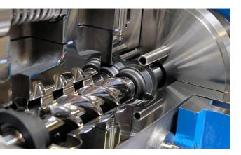
The pump only requires two signals - a temperature transmitter on the isolation shell to provide a startup interlock to ensure proper pre-heating temperature, and a PT100 on the casing to ensure the maximum temperature for the pump is not exceeded. Otherwise no additional accessories are required, and the product is not contaminated by any auxiliary fluids.
